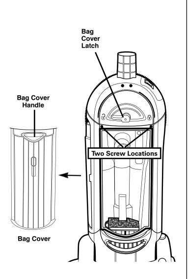
Remove bag cover from unit to expose the two screw installation locations. Release the bag cover by rotating the bag cover latch to the left. Pull out and up on the bag cover handle to remove bag cover from unit.
